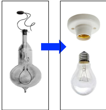
Hazardous Wire Installs For Bulbs Safety Mandatory Standardization of Bulbs Screw Installs
